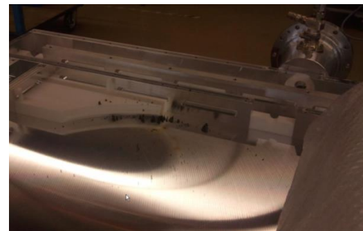
Ferrite chips and burning marks close to port 1.
