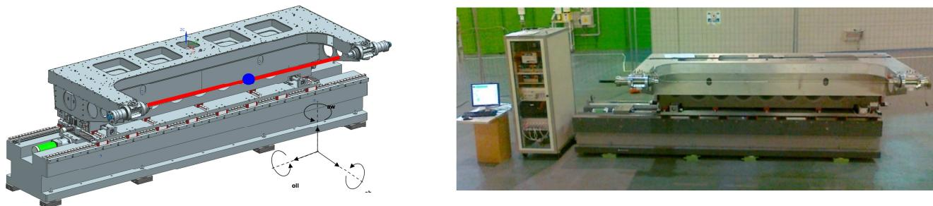
**Figure 1:** Design and picture of the new Hall probe bench prototype built at CELLS.
